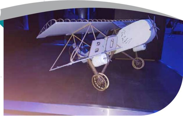
The classic twin wing glider was designed by specialized computer programs. The team took care of the exact details of the object by studying its structural designs and drawing from specialized sites. The team then combined cork and wood using laser cutting machine as well as taking advantage of the 3D printer to design some parts such as wheels.
